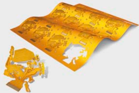
Separation of individual interconnect devices and populated circuit boards from larger panels.
