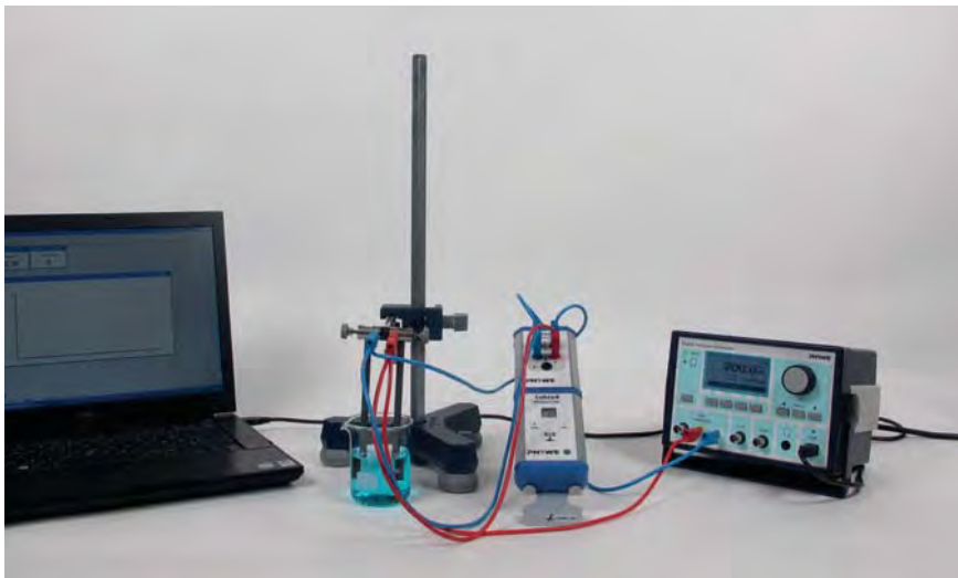
Current/voltage characteristics of an aqueous copper sulphate solution conducted with graphite electrodes and copper wires.
