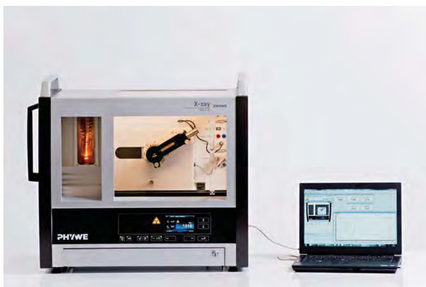
Intensity of the X-ray spectrum of copper as a function of the glancing angle theta: NaCl monocrystals with [111] crystal orientation as Bragg analyser.
