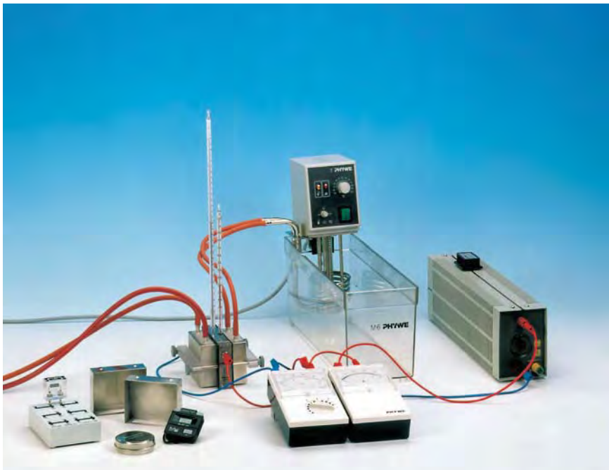
Electrical power generated as a function of the temperature difference.
