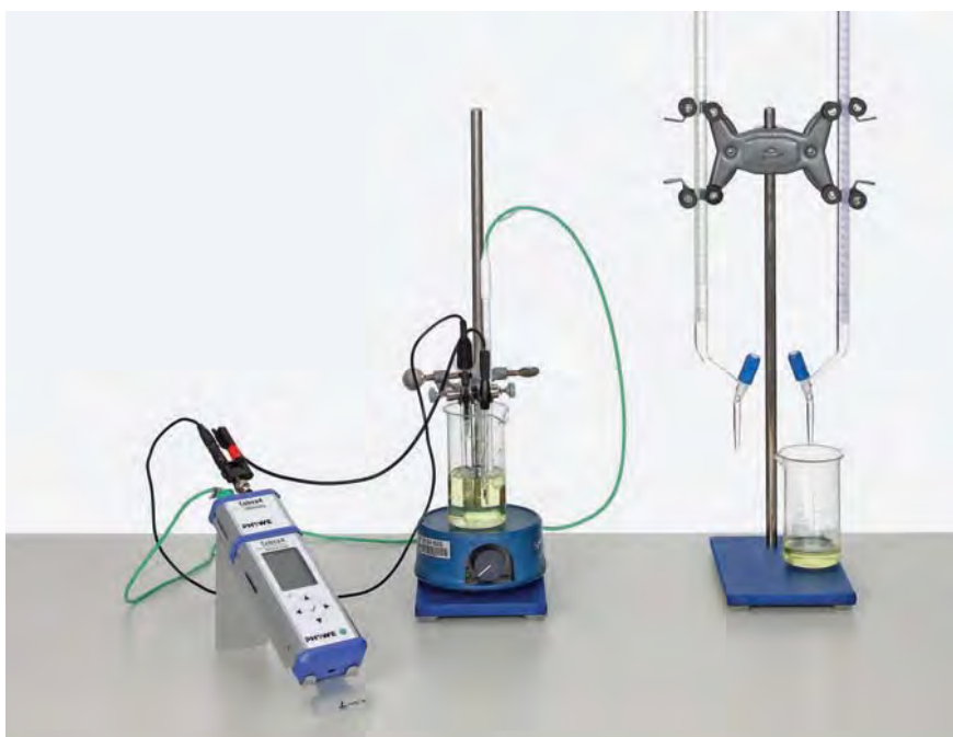
Verification of the Nernst equation for the \text{Fe}(\text{CN})_6^{4-} , \text{Fe}(\text{CN})_6^{3-} Pt redox electrode.
