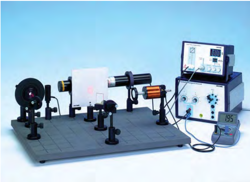
Formation of circular interference fringes.
