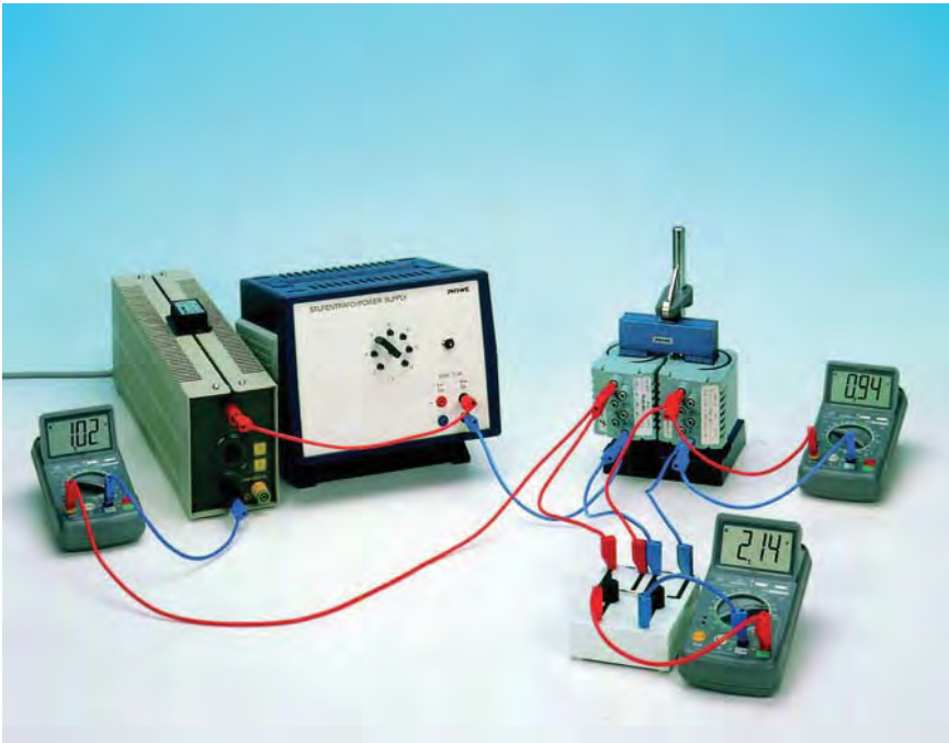
Secondary short-circuit current of the transformer as a function 1. of the number of turns in the secondary coil, 2. of the number of turns in the primary coil.
