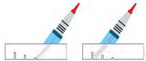
Reflection of an ultrasound beam at a small crack (left) and at a deep crack (right).
