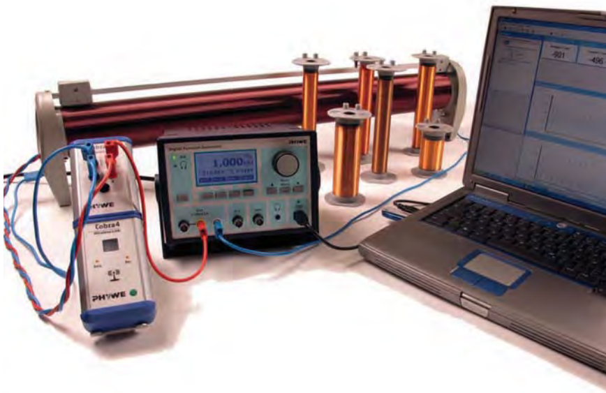
Induced voltage as a function of current for different coils.
