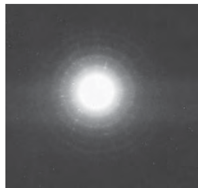
Debye-Scherrer pattern of a powdered sample of NaCl. Thickness of the sample: 0.4 mm. Exposure time: 2.5 h. Mo X-ray tube: U_a = 35 kV; I_a = 1 mA.
