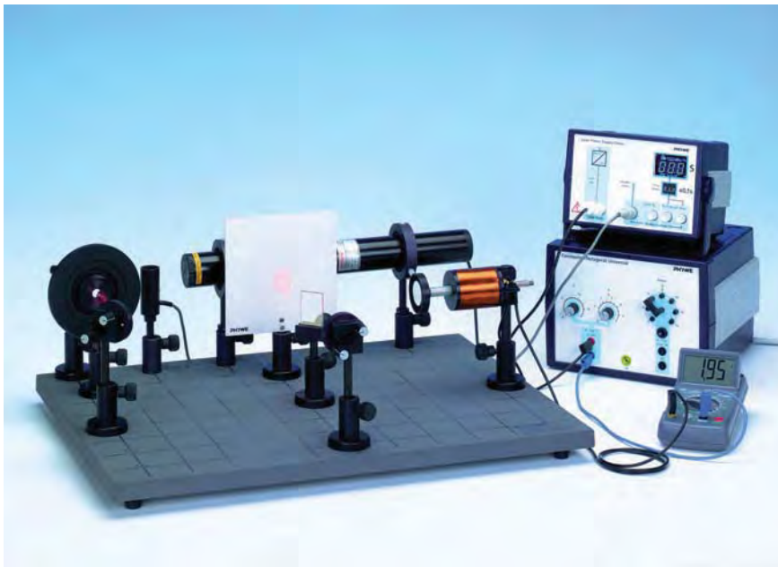
Formation of circular interference fringes.
