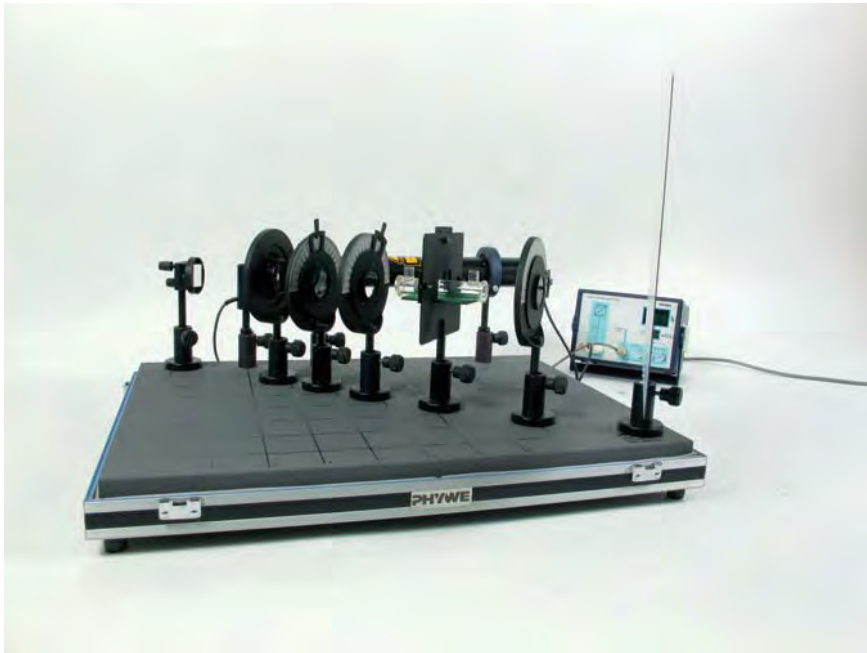
Working principle of the half shadow polarimeter.
